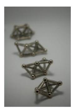
The magnetic "stick and ball" construction toys first used to understand entropy, or all the possible cluster structures that could be formed from a given number of particles. Credit: Vinothan Manoharan, Harvard School of Engineering and Applied Sciences
