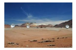
Three ALMA antennas linked together as an interferometer for the first time, on the 5,000 m altitude plateau of Chajnantor. Having three antennas observing in unison makes it possible to correct errors that arise when only two antennas are used, thus paving the way for precise images of the cool Universe at unprecedented resolution. Credit: ALMA (ESO/NAOJ/NRAO)
