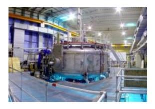
The Levitated Dipole Experiment (LDX) reactor is housed inside a 16-foot-diameter steel structure in a building on the MIT campus that also houses MIT's other fusion reactor, a tokamak called Alcator C-mod.
