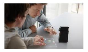
Holographic refers to the method Light Blue Optics uses to create twodimensional images by transforming original images into sets of diffraction patterns that are shown on a micro-display and then illuminated by laser light. Diffraction patterns are used because of their high efficiency, since they direct light to where it is needed rather than indiscriminately.
