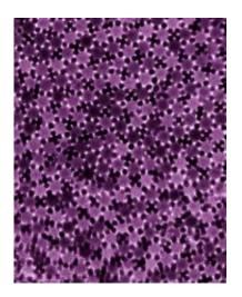
TEM showing the two-dimensional dodecagonal quasi-crystalline structure selfassembled from 5-nm Au and 13.4-nm Fe3O4 nanoparticles.
