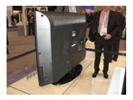
TV images are displayed by using WHDI (Wireless Home Digital Interface), a high-speed communication standard for wirelessly transmitting high-definition images. This leaves the back of the TV completely wire free.
