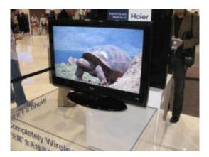
Wireless content is transferred by a system called Wireless Home Digital Interface (WHDI). Using a 5GHz frequency band it can transfer uncompressed 1080p 60Hz video to the TV.
