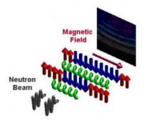
The magnetic field is used to tune the chains of spins to a quantum critical state. The resonant modes ("notes") are detected by scattering neutrons. These scatter with the characteristic frequencies of the spin chains. Credit: Tennant/HZB
