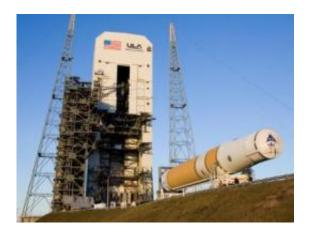
On Cape Canaveral Air Force Station in Florida, the core stage of a Delta IV rocket arrives at Launch Complex 37. The rocket's core stage is the first stage mated to the second stage. This United Launch Alliance Delta IV rocket is slated to launch GOES-P developed by NASA for NOAA. Credit: NASA/Jack Pfaller
