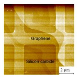
Graphene, only one atom thick, climbs terraces on the surface of a silicone carbide substrate. This picture of a graphene device was taken with an atomic force microscope by NPL's Dr Olga Kazakova
