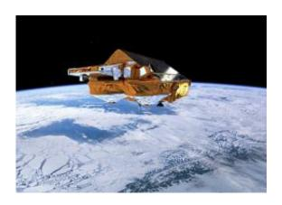
ESA's Earth Explorer CryoSat mission is dedicated to precise monitoring of the changes in the thickness of marine ice floating in the polar oceans and variations in the thickness of the vast ice sheets that overlay Greenland and Antarctica. Credits: ESA/AOES Medialab
