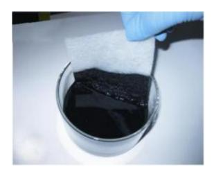
Fabrics treated with this new electrically-conductive ink may power a new generation of futuristic clothing that charges iPods, cell phones and other electronics. Credit: American Chemical Society
