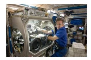
Astronaut Bob Thirsk installs the IVIDIL bench into the microgravity science glovebox on board the International Space Station. The bench is part of SODI-IVIDIL, a European experiment which features Canadian contribution from mechanical and industrial engineering professor Ziad Saghir. Photo credit: NASA.
