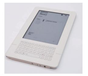
• Jinke SiPix panel e-reader uses SiPix panels for the A6 and A9 readers. Both the 6 and 9 inch devices have 16 levels of grayscale, WiFi a/b/g, and optional 3G. Supports formats FB2, EPUB, PDF, most image formats, and MP3. The 6-inch (600 x 800) device has 2GB of storage, an SD slot, and an accelerometer. The 9-inch (1024 x 768) device has up to 4GB storage. The A6 retails for \$275 and the A9 for \$330; both should be available in March.
