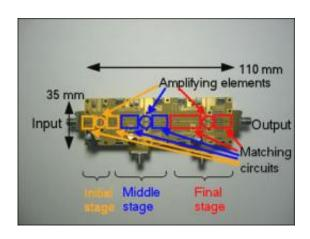
NTT DOCOMO announced today that it has developed a prototype multi-band power amplifier that accommodates eight frequency bands between 700 MHz and 2.5 GHz, paving the way for lightweight, all-in-one mobile phones capable of standalone wireless communications of different standards, including the forthcoming extra-fast LTE standard as well as existing W-CDMA and GSM.
