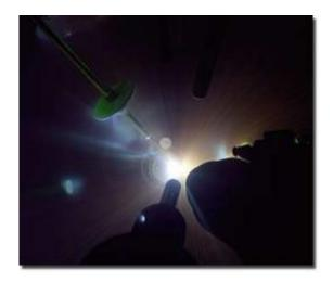
Time-integrated photograph of an OMEGA laser shot (43633) to measure highpressure diamond strength. The diamond target is at the center, surrounded by various diagnostics. The bright white light is ablated plasma, and radial yellow lines are tracks of hot target fragments very late in time. Photo by Eugene Kowaluk/LLE
