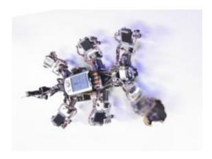
Following the principle of chaos control, the robot produces regular leg movements when walking normally. In addition, it can use the uncontrolled chaotic movement pattern to free itself when its leg is trapped in a hole. Image: Network Dynamics Group, Max Planck Institute for Dynamics and Self-Organization
