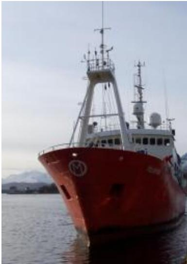
The Norwegian weather ship Polarfront is equipped with a battery of instruments to measure wind speed, humidity and carbon dioxide. Credit: Margaret Yelland (NOCS)
