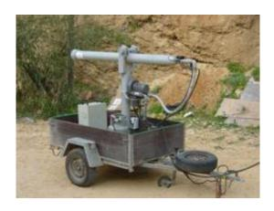
The Thunder Generator produces shock waves that result in a loud sonic boom and extreme air pressure, which can be heard and felt by people up to 100 meters away. Image credit: Army Tec.
