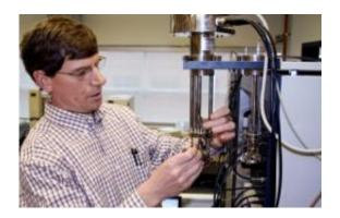
Steve Martin of Iowa State University and the US Department of Energy's Ames Laboratory loads ion-conducting glass, a solid electrolyte used in batteries, into an impedance spectrometer that measures ion conductivity. High conductivity is required for the electrolytes in batteries. Credit: Photo by Patrick Herteen/Engineering Communications/Iowa State University
