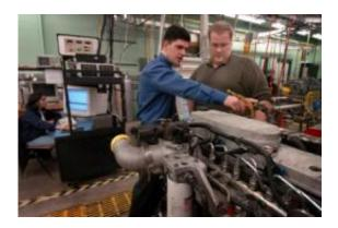
Gregory M. Shaver, from left, an assistant professor of mechanical engineering at Purdue, and graduate student David Snyder discuss how to modify a commercial diesel engine with a new technique that promises to reduce emissions of nitrogen oxides for engines running on biodiesel. Graduate student Gayatri Adi (background) reviews software algorithms needed for the new technology.
