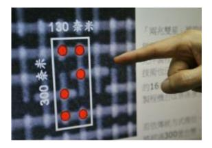
An electronic image shows six transistors installed in a space measuring 300 nanometres by 130 nanometres on a microchip developed by State-backed National Nano Device Laboratories.
