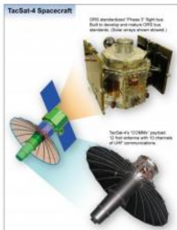
TacSat-4 illustration showing solar arrays stowed and showing COMMMx payload. Credit: Naval Research Laboratory
