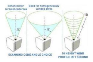
Leosphere's Windcube can measure the wind profile at ten programmable measurement heights in the range either 40-200 m or 100-5000 m vertically above the point of measurement. Because wind circulation can differ from site to site, the measurement can be taken with either a 15° or 30° scanning cone angle. Credits: Leoshere
