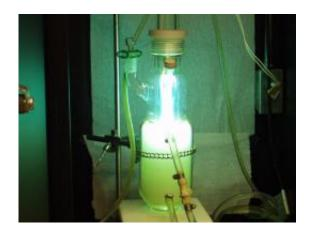
By exposing a colloidal suspension of zinc sulfide and sodium sulfide to UV light, the research team has been able to reproduce many steps of a primitive metabolic cycle. Image Credit: Marcelo Guzman/Harvard University
