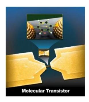
Engineers adjusted the voltage applied via gold contacts to a benzene molecule, allowing them to raise and lower the molecule's energy states and demonstrate that it could be used exactly like a traditional transistor at the molecular level. Credit: Hyunwook Song and Takhee Lee
