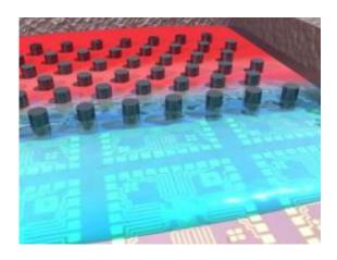
Blood is filtered and transferred to nanosensors on a chip, which can detect and measure cancer biomarkers. Credit: Mark Reed/Yale University
