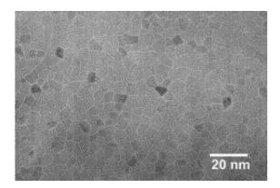
An electron microscopy image of titanium nitride, on which the effect of superinsulation was first observed.
