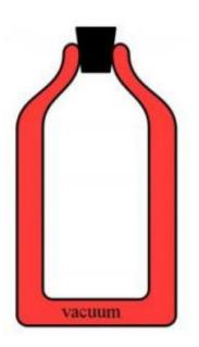
In a typical thermos, a vacuum is used to reduce heat transfer. Scientists have found that layers of photonic crystals in a vacuum can reduce the thermal conductance to about half that of a pure vacuum. Credit: Wikimedia.
