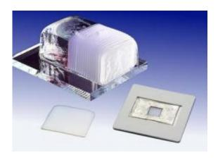
The glass dosimeter detects the buildup of pollutant gases in picture cases. Credit: K. Dobberke/Fraunhofer ISC
