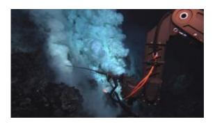
The Jason remotely-operated vehicle (ROV) samples fluid at an eruptive area near the summit of the West Mata Volcano, May 2009. The fluid sampling "wand" is approximately three feet long. (Image courtesy of NSF, NOAA, and WHOI Advanced Imaging and Visualization Lab)
