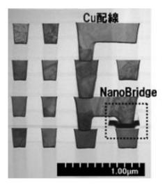
NEC Corporation, in collaboration with the National Institute of Materials Science, today announced the successful integration of NanoBridge, a solid electrolyte non-volatile crossbar switch, in Cu interconnects placed on CMOS logic. This development enables the realization of high performance non-volatile programmable logic at a low cost.
