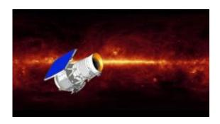
The Wide-field Infrared Survey Explorer mission will survey the entire sky in a portion of the electromagnetic spectrum called the mid-infrared with far greater sensitivity than any previous mission or program ever has.
