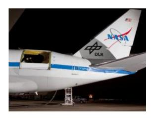
The rear fuselage of the Stratospheric Observatory for Infrared Astronomy's 747SP is illuminated during telescope testing operations in preparation for aircraft and science checkout flights. The telescope cavity door is open with the lower flexible door partially extended. (NASA Photo / Tom Tschida)
