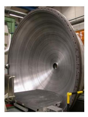
A full-scale spherical tank dome measuring 18 feet in diameter was produced from high-strength 2195 aluminum-lithium using twin manufacturing processes.
