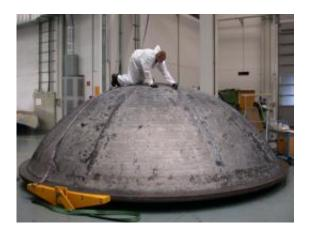
The spherical tank dome was manufactured from a flat plate "blank" made of the 2195 alloy. The blank was constructed by friction stir welding together two commercial off-the-shelf plates in order to produce a large starting blank. The welded plate blank was then spun formed to create the single-piece tank dome. (MT Aerospace)
