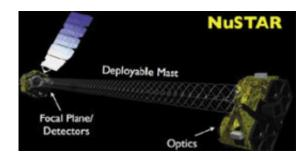
NuSTAR with primary instrument components labeled. Image credit: NASA
