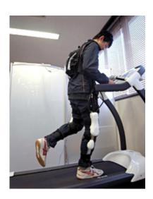
The motorized knee has a small motor that helps flex the knee, a sensor that detects the degree of flexing of the knee, and a safety lever.
