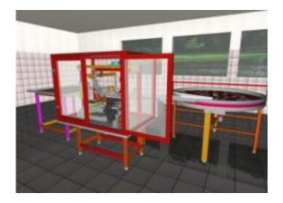
Trainees use a computer to operate this virtual handling system for biological compounds. They can transport Petri dishes with bacteria cultures over a conveyor, control grippers and take samples. Credit: Fraunhofer IFF
