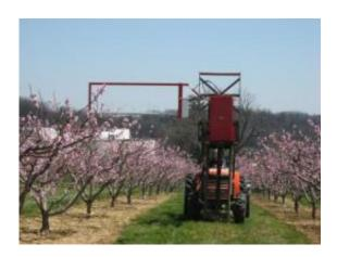
The horizontal prototype of a string thinner is designed to thin peach blossoms in orchards trained to open-center or vase systems. Credit: Photo courtesy of Tara Baugher
