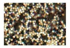
Reflection optical microscope image of a dried suspension of the discs prepared via magnetron sputtering and optical lithography.
