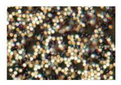
Reflection optical microscope image of a dried suspension of the discs prepared via magnetron sputtering and optical lithography.
