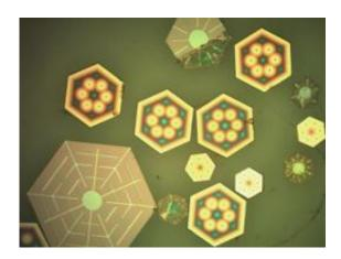
These are representative thin crystalline-silicon photovoltaic cells -- these are from 14 to 20 micrometers thick and 0.25 to 1 millimeter across. Credit: Murat Okandan
