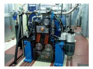
This test engine is the centerpiece of a project called NEMo, a German acronym meaning "lowest emission diesel engine for trucks." Researchers at the Technische Universitaet Muenchen have used it to demonstrate simultaneous reduction of nitrogen oxides and soot, without resorting to a catalytic converter. Credit: Sebastian Pflaum, TU Muenchen
