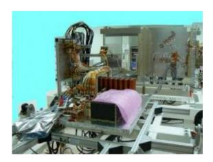
The Galileo in-orbit verification engineering model satellite platform, showing the power subsystem undergoing testing at Thales Alenia Space, Rome. Credits: ESA / Thales Alenia Space Italia
