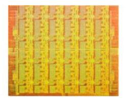
Single Chip Cloud Computer has 48 Intel cores and runs at as low as 25 watts
