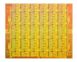
Single Chip Cloud Computer has 48 Intel cores and runs at as low as 25 watts
