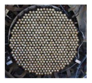
A Veritas "camera" made of photomultiplier tubes detects the brief flashes of light generated by a cascade of charged particles produced when high-energy gamma rays strike Earth's atmosphere. Image: Frank Krennrich
