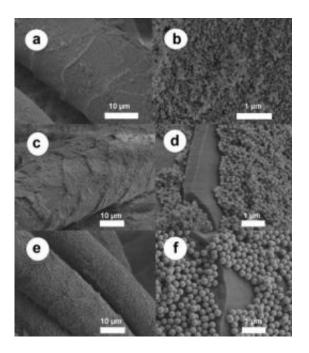
These images from an electron microscope show wool fibers coated with the silica nanoparticles that may improve wool's qualities. Credit: American Chemical Society
