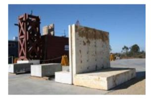
Engineers tested two types of retaining wall systems -- one without a sound barrier (foreground) and one with a sound wall (background) during a series of rigorous simulated earthquake tests at UCSD's Englekirk Structural Engineering Center, which has the largest outdoor shake table in the world. Credit: UC San Diego
