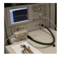
Verifying the performance of vector network analyzers—devices that check how components used in cell phones, radios and satellites transmit signals—has gotten a lot easier and faster with this plug-in device and accompanying software developed by NIST. A process that once took hours or days can now be done in minutes. Credit: Burrus, NIST
