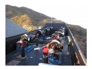
The MEarth (pronounced "mirth") Project is an array of eight identical 16-inch-diameter RC Optical Systems telescopes that monitor a pre-selected list of 2,000 red dwarf stars. Each telescope perches on a highly accurate Software Bisque Paramount and funnels light to an Apogee U42 charge-coupled device chip, which many amateurs also use. Credit: Dan Brocious, CfA
