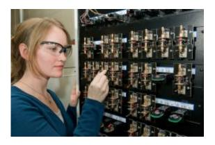
Argonne researcher Lynn Trahey loads a coin-sized cell on a testing unit used to evaluate electrochemical cycling performance in batteries. Photo by Wes Agresta.
