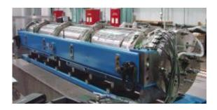
The completed long quadrupole shell magnet (LQS01) in the Building 77A assembly area of Berkeley Lab's Engineering Division.
